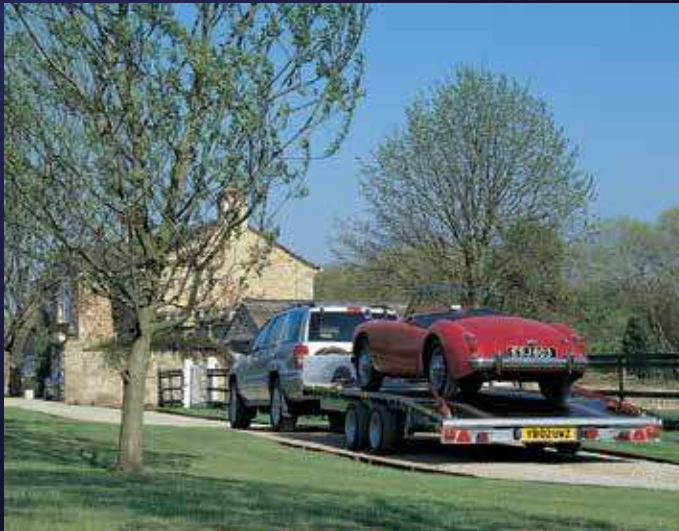
LM167/B with optional headboard, skids, electric winch, propstands and lashing rings
